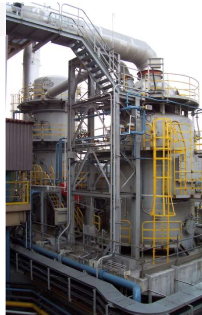
Off-Gas Cleaning Plant of a Copper-Slag Cleaning Furnace in Chuquicamata (Chile)
