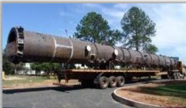
Fractional Tower + Trays + Stairs and Platforms - ASME Sec.VIII-DIV.1 - OS: 25.469/2.009 Øi 1.900 X 29.241 mm - Weight: 25,5 Ton. Material: SA-516 Gr.70
