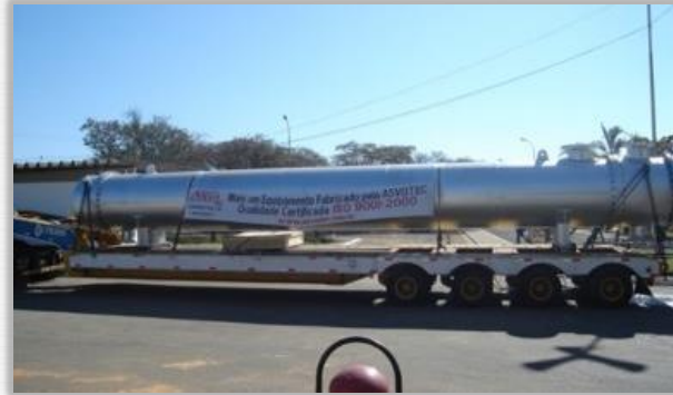
Depropanizer Condenser – AEM - PB/REVAP/SP Øi 1.450 X 14.530 mm - Weight: 45,0 Ton. Material: SA-516 Gr.60 /SA-179/SA-516 Gr.70/SA-105
