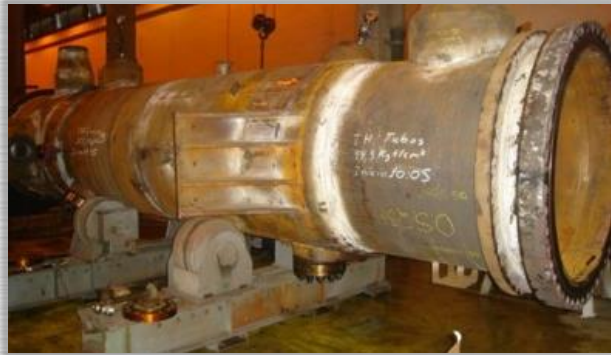
Heat Recovery Boiler – NEN PB/FAFEN/Laranjeiras/SE Øi 1.194 X 7.620 mm - Weight: 31,6 Ton. Material: SA-516 Gr.70 /SA-213-Gr. T11/SA-182-Gr.11-CL.2
