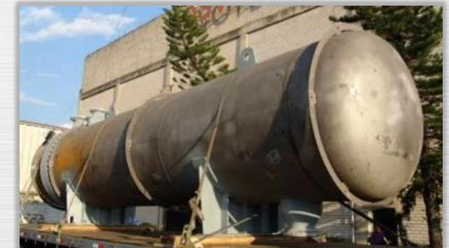
Cargo and Bottom Exchanger – BEU PB/RPBC/SP – Hydro / Treatment Unit UT / HTD Øi 1.610 X 8.260 mm - Weight: 29,0 Ton. Material: SA-516 Gr.60 /SA-268 TP405/SA-105+CLAD 410 S
