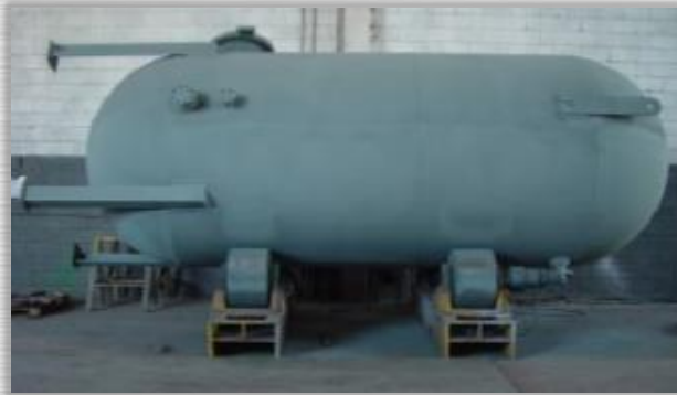
Lung Vessel for Nitrogen - OS: 23.787/2.006 Øi 2 200 x 6.400 mm – Weight: 10,3 Ton
