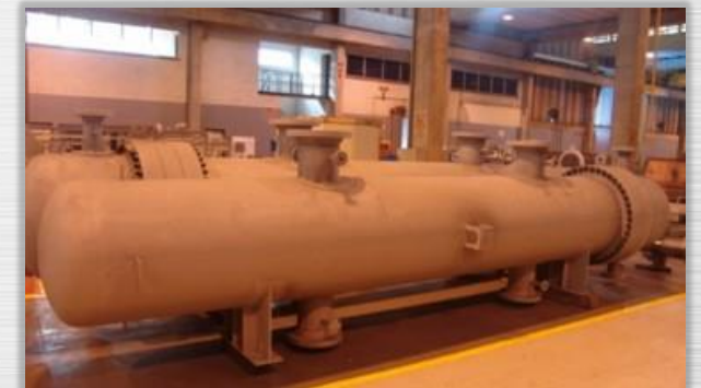
Stabilizer Reboiler – BHU PB/RPBC/SP – Catalytic Reform Unit (URC) Øi 1.025 X 8.008 mm - Weight: 15,4 Ton. Material: SA-516 Gr.70 /SA-179/SA-105 N
