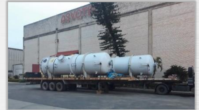
VRU 1st Stage Suction Scurrber - OS: 30.340/2.019 Clad 316L Øi 2 300 x 7.500 mm – Weight: 16,0 Ton
