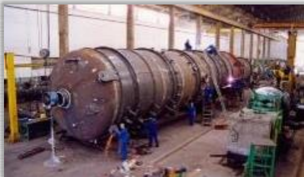
Pre Vacuum Tower + Trays + Stairs and Platforms - ASME Sec.VIII-DIV.1 - OS: 21.000/2.002 Øi 4.500 X 31.040 mm - Weight: 117,0 Ton. Material: SA-516 Gr.60 + SA-240-317L (CLAD)
