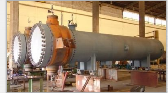
Preheater – DFU - PB/RPBC/SP Øi 1.321 X 7.984 mm - Weight: 25,5 Ton. Material: SA-516 Gr.60 /SA-268 TP405/SA-266 Gr. 4/SA-105
