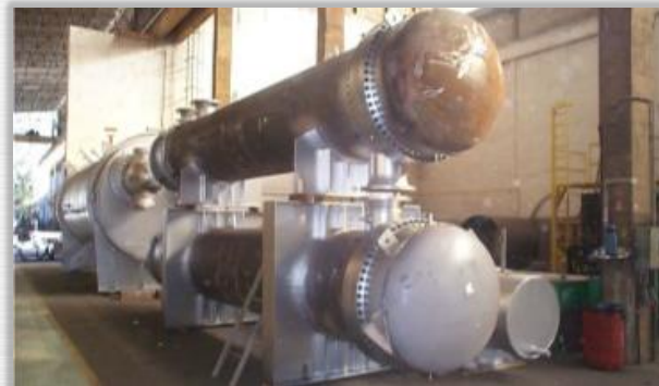
Debutanizer Petrol Cooler – AES PB/REDUC/RJ – UFCC REVAMP Unit (U1250) Øi 1.105 X 7.365 mm - Weight: 15,8 Ton. Material: SA-516 Gr.60 /SA-179/SA-105
