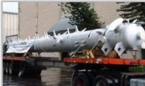
Regenerative Tower + Trays + Stairs and Platforms - ASME Sec.VIII-DIV.1 - OS: 24.063/2.007 Øi 1.000 X 18.636 mm - Weight: 13,5 Ton. Material: SA-240-304L/SA-240-316L
