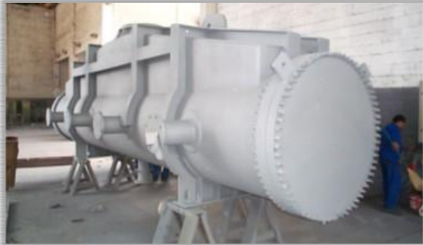
Vacuum System Pre-Condenser PB/RPBC/SP Øi 1.143 X 6.932 mm – Weight: 16,0 Ton. Material: SA-516 Gr.60 /SA-179/SA-516 Gr. 70/SA-105
