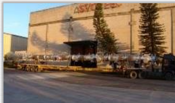
Regenerative Tower + Trays + Stairs and Platforms - ASME Sec.VIII-DIV.1 - OS: 25.722/2.01 Øi 915 X 33.050 mm - Weight: 29,6 Ton. Material: SA-516 Gr.70 + SA-240-316L (CLAD)
