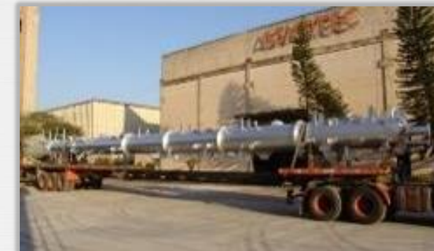
Absorbing Tower + Trays + Stairs and Platforms - ASME Sec.VIII-DIV.1 - OS: 25.721/2.010 Øi 915 X 24.900 mm - Weight: 21,7 Ton. Material: SA-516 Gr.70 (B Class H2S)
