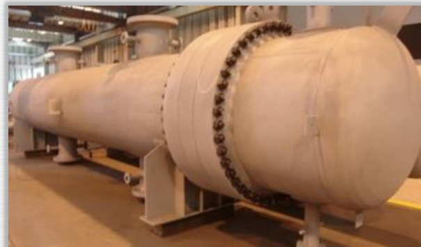
H2S Striker Reboiler – BHU PB/RPBC/SP - Catalytic Reform Unit (URC) Øi 1.100 X 8.083 mm Weight: 25,5 Ton. - Material: SA-516 Gr.70 /SA-179/SA-105 N
