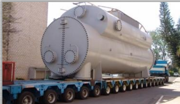
Surface Condenser SIEMENS - PB/RFAP/ Power Generator Øi 3.700 X H 5.350 X 14.741 mm - Weight: 152,0 Ton. Material: SA-285 Gr.C /SB-111-C44300/SA-516 Gr. 70/SA-105
