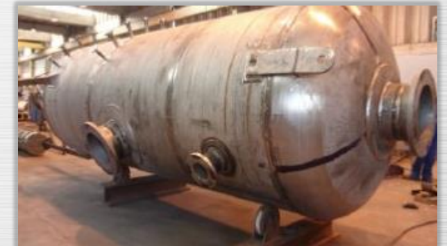
Compressor Suction Vessel - OS: 24.045 Øi 1.700 X 6.245 mm - Weight: 3,6 Ton
