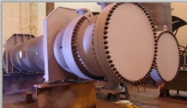
Heat exchanger – AES PB/RPBC/SP – UNA 25 Unit (URC) Øi 1.143 X 7.500 mm - Weight: 19,6 Ton. Material: SA-516 Gr.60 /SA-179/SA-516 Gr.70/SA-105
