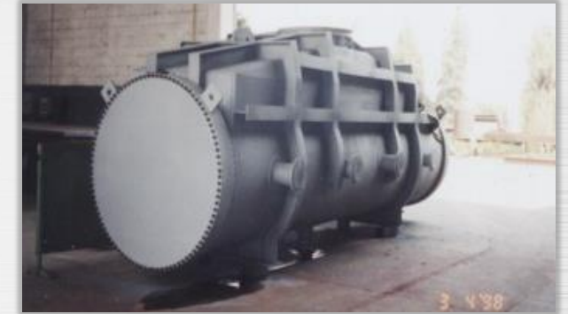
Vacuum System Intercondenser PB/RPBC/SP Øi 1.676 X 7.126 mm - Weight: 31,4 Ton. Material: SA-516 Gr.60 /SA-179/SA-516 Gr. 70/SA-105
