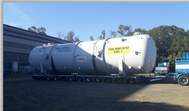
N1 LP Flare Knock-Out Drum OS: 30.343/2.019 Øi 4.600 X 18.000 mm - Weight: 66 Ton
